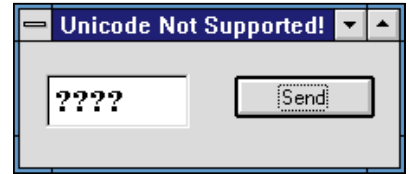
FIGURE 2 No Unicode Support In Visual Basic. Apparently for compatibility with Windows 95, Microsoft decided to explicitly disable NT's native Unicode support. If a true Unicode string is sent to an intrinsic VB control, the control displays it as a series of question marks, regardless of which font is selected into the control.
